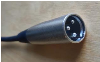
Male XLR plug (i.e. the pins stick out)
